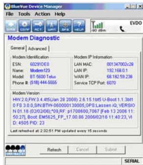
BlueVue Device Manager For initial setup and configuration
